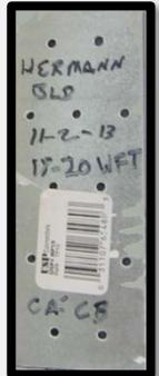
To use the WFT gauge, place the gauge directly on the wet area just sprayed as described above (see figure 2). The notches will indicate the measured film thickness. For example, if the 18 mil notch is wet and the 20 notch is dry, then the wet measured thickness is 18 mils.
