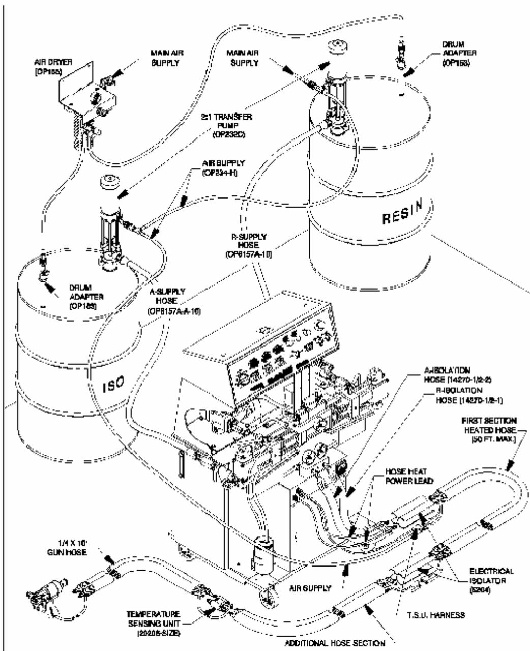
Typical spray polyurethane foam equipment setup
