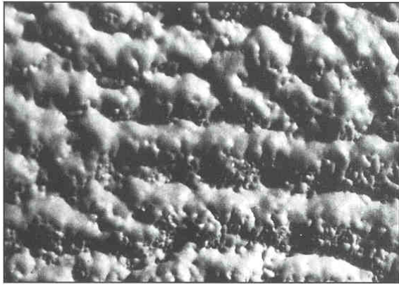
Photo 4 Polyurethane Foam Texture Rippling – Verge of Popcorn
