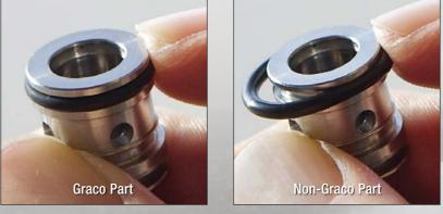
After spending the same amount of time submersed in solvent, the Graco O-ring (left) still fits snugly, protecting the side seal, while the non-Graco O-ring (right) expanded in diameter and swelled in cross section.
