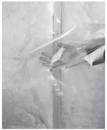
This product can be used in place of traditional vapor retarders with unfaced fiber glass insulation to provide an insulation system that is ideal in some of the more severe climate condition areas in terms of both temperature and humidity. In addition, MemBrain may be installed as an interior air barrier system combined with recommended tapes and sealants.
