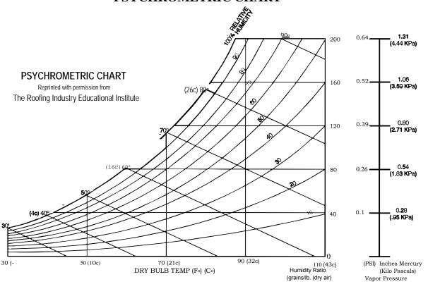
The psychrometric chart is used to determine and correlate the following properties of humid air:
