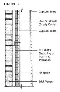
Steel stud cavity wall with interior and exterior gypsum, uninsulated stud cavity, and no air/vapor retarder. The designer may want to consider sealing the external joints of the foam by taping or caulking.
