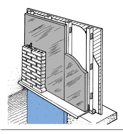
THERMAX Sheathing, with aluminum facers on both sides, features improved fire performance due to special chemical modifications of its foam core, making it an ideal choice for many types of facilities. THERMAX Sheathing can be installed exposed to the interior without a thermal barrier in many applications.
