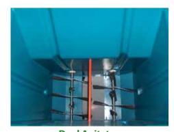
**Dual Agitators**Designed for Constant Material Flow
