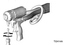
12. Disengage piston safety lock (L). See **Piston Safety Lock**, page 20.
