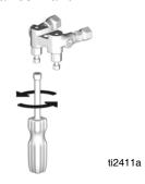
2. Connect A (ISO) and B (RESIN) fluid hoses to fluid manifold.
