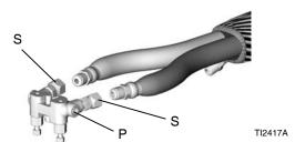
5. Apply thread sealant to plugs (12c), elbows (50\*), and male threads of fluid inlet swivels (S). Install elbows (50\*) in optional fluid inlets (P), facing down. Install swivels (S) in elbows. Be sure to install A swivel (smaller) in A side. Install included plugs where swivels were located. Torque all parts to 235-245 in-lb (26.6-27.7 N•m).
