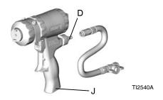
Reattach fluid manifold. Reconnect air. Return gun to service.
