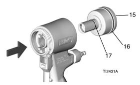
7. Liberally lubricate piston o-rings. Reinstall piston. Shaft is keyed for proper assembly. Push firmly to seat piston.
