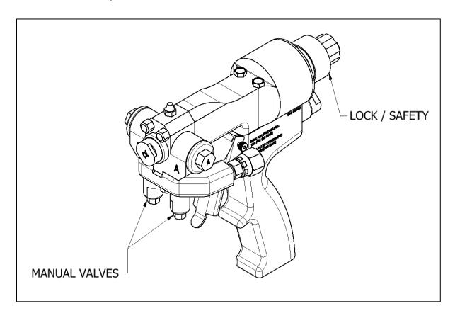
WARNING! Before proceeding with any maintenance work on the Xtreme Gun, trigger the gun to remove internal material pressure, ensure the Manual Valves are CLOSED, ensure the Gun Lock is in the LOCKED position, and SHUT OFF/DISCONNECT the air supply. It is recommended to remove the Gun from the Coupling Block.
