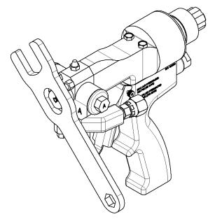
CAUTION! Use wooden or plastic tools or a brass brush for cleaning. Do not use metal or abrasive tools that can scratch or damage the contact surfaces.
