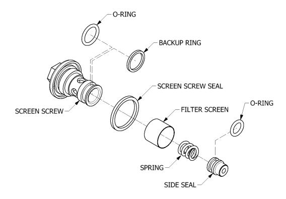
CAUTION! To avoid possible contamination by the residual chemical inside the Gun do not interchange the Isocyanate (A) parts with the Polyol (R) parts. The Isocyanate (A) side is identified with an (A) on the Screen Screw Head and the Polyol (R) side is marked with an (R) on the Screen Screw Head. The Gun Block is also marked with (A) and (R) designation.
