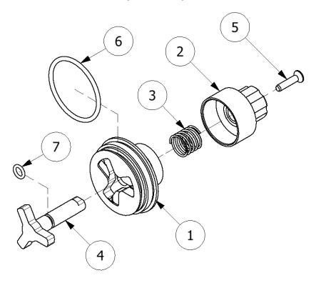
**NOTE:** WHEN ASSEMBLING BE SURE TO APPLY GREASE TO **ALL** O-RINGS. THIS ENSURES GOOD PERFORMANCE AND REDUCES RISK OF GUN MALFUNCTION.
