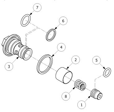
**NOTE**: WHEN ASSEMBLING BE SURE TO APPLY GREASE TO **ALL** O-RINGS. THIS ENSURES GOOD PERFORMANCE AND REDUCES RISK OF GUN MALFUNCTION.
