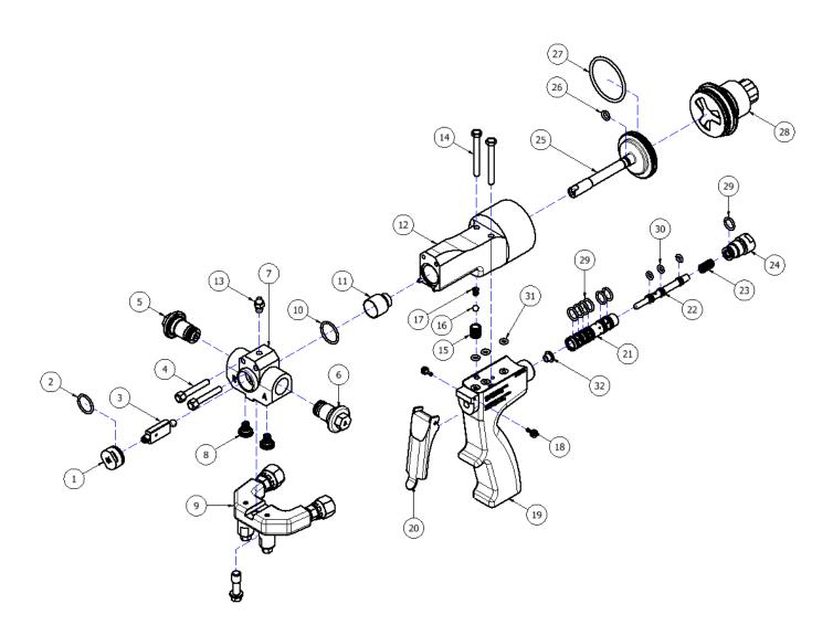
**NOTE:** WHEN ASSEMBLING BE SURE TO APPLY GREASE TO **ALL** O-RINGS. THIS ENSURES GOOD PERFORMANCE AND REDUCES RISK OF GUN MALFUNCTION.
