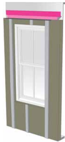
Step 14: Install furring over ROCKWOOL COMFORTBOARD™ 80 insulation.
