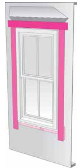
Step 7: Back-caulk window. Apply sealant at jambs and head; do not apply to sill to allow for drainage. Or, caulk can be applied to window nailing flange prior to installation.
