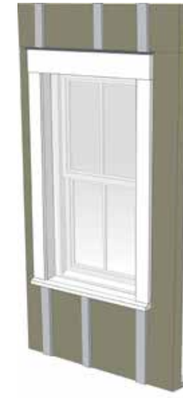
Step 19: Trim installed at head and jambs; sloped cap flashing (shown) installed over lower trim at head of window.
