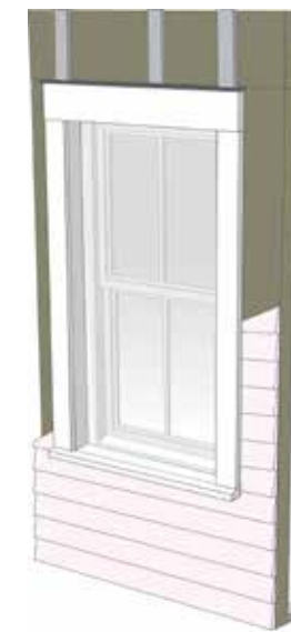
Step 19: Trim installed at head and jambs; sloped cap flashing (shown) installed over lower trim at head of window.
