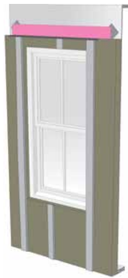
Step 13: Install ROCKWOOL COMFORTBOARD™ 80 insulation.
