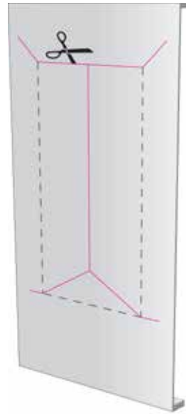
Step 2: Modified "I" cut in housewrap over framed opening (dashed line above)
