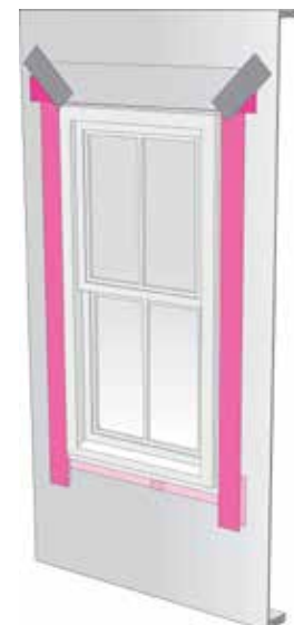
Step 9: Install jamb flashing; extend minimum 1" above head nailing flange and a minimum 3" below sill nailing flange.
