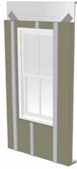
Step 14: Install furring over ROCKWOOL COMFORTBOARD™ 80 insulation.
