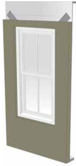
Step 13: Install ROCKWOOL COMFORTBOARD™ 80 insulation.
