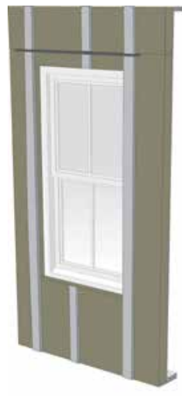
Step 15: Outward leg of cap flashing extends past face of trim (to be added in Step 19).
