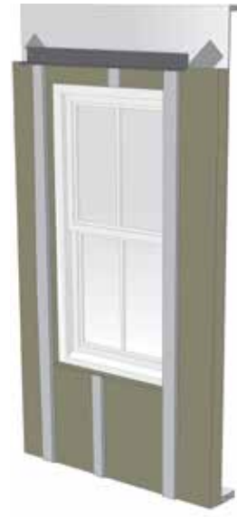
Step 15: Outward leg of cap flashing extends past face of trim (to be added in Step 19).
