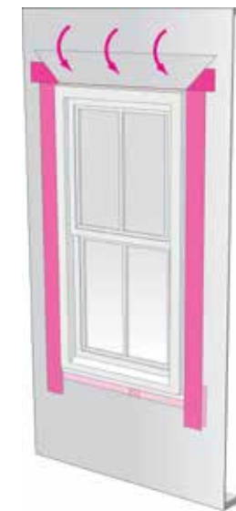
Step 8: Install window plumb, level and square per manufacturer's instructions.
